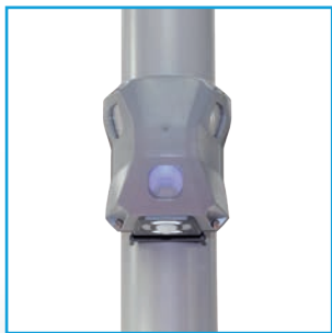
Motion Sensor triggers up 1 to 10 devices. Detects pedestrians, cyclists and cars range (range: 2.5 -75 mph) Range: up to 15m on each side, 9m front and 3m behind at a mounting height of 5m (max).
