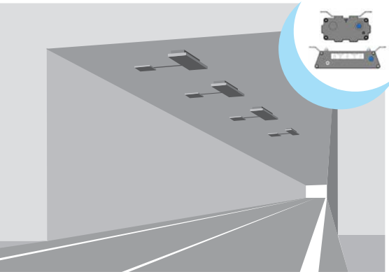
Example of assembly with GBOX separated from the luminaire.
