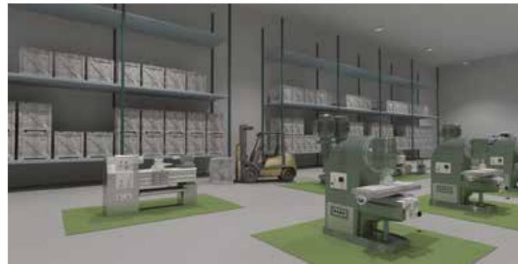
Representation of a sample industrial building with objects, using direct light high bay luminaires.
