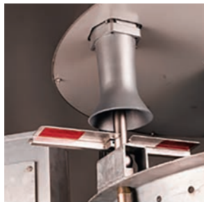
Positive fail-safe latching
